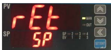
Figure 1: Set retransmitting output values to be based on SP values
